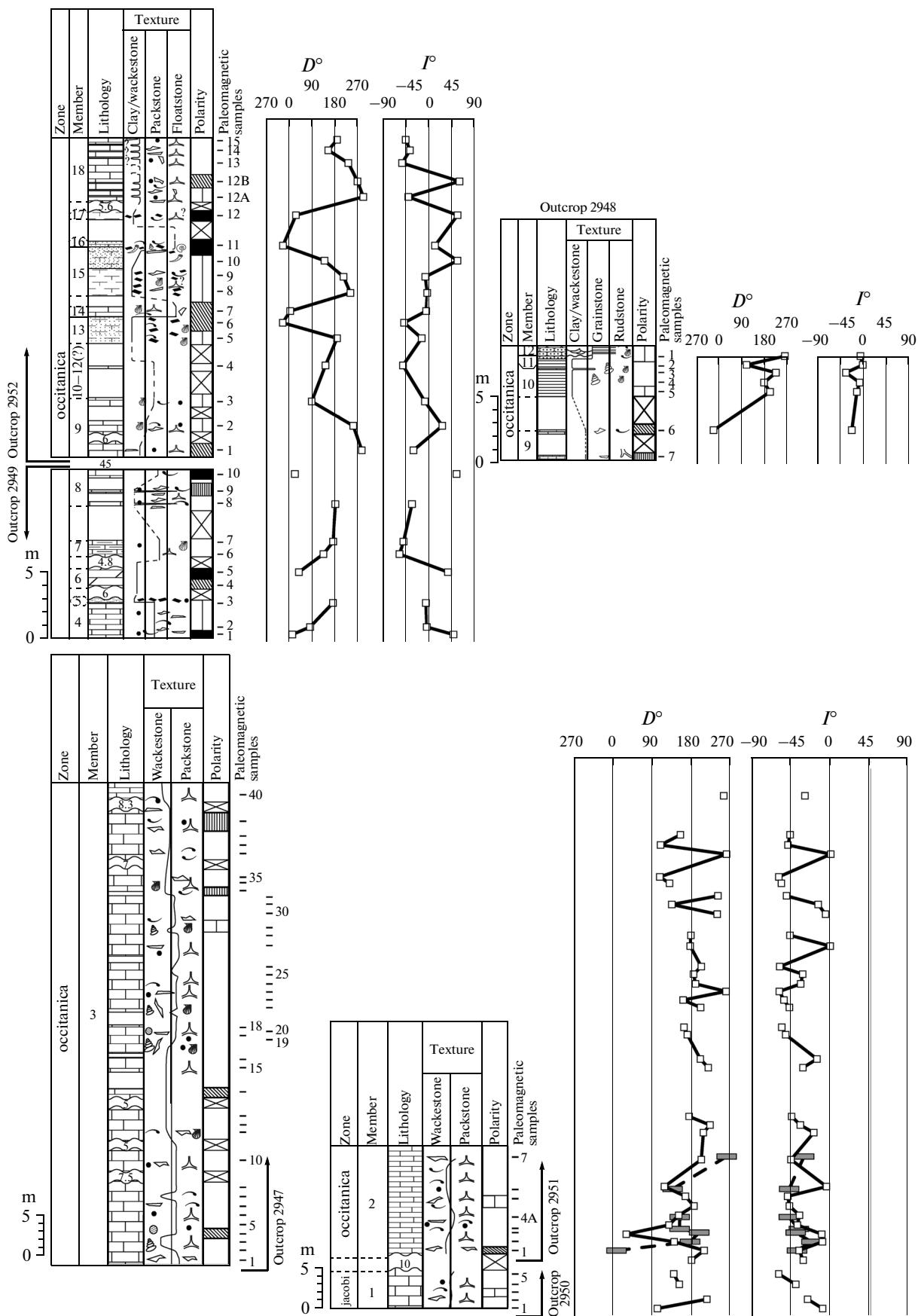
Fig. 3. Lithological-sedimentological and paleomagnetic data on outcrops 2947–2952. For legend, see Fig. 4.
