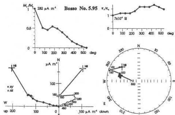
Fig. 2. Bosso Valley, Umbria, central Italy, typical properties of normally polarized samples.
