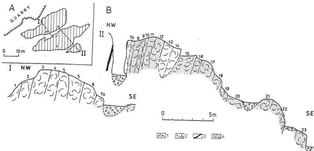
Fig. 14. Cross-section through the Rogoża Klippes (after Kutek and Wierzbowski, 1986): A - sketch map of the klippes showing the lines of the section, B - cross-section through the klippes, 1 - sparry coquinas (Lower - Middle Tithonian), 2 - micritic coquinas, also micritic limestones in neptunian dykes (uppermost Tithonian - Middle Berriasian), 3 - crinoidal limestones in neptunian dyke (?Valanginian), 4 - rubble.
